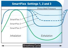
SmartFlex offers three pressure reduction settings that will automatically reduce the pressure generated by the IntelliPAP upon exhalation and raise the pressure back up to prescribed pressure at the onset of inspiration. The settings correlate to an exact cm  $H_2O$  pressure drop – so a setting of 1 = 1 cm  $H_2O$  drop in pressure during exhalation.
